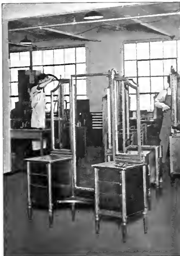
Frame of vanity dresser assembled ready for finishing.
